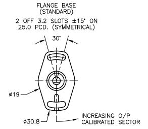
SHAFT FLAT ALIGNED WITH REFERENCE MARK IN BASE AT MID TRAVEL ±5°
